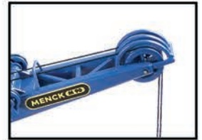
03. lead the grabber ropes (1) and (3) across the roll head
